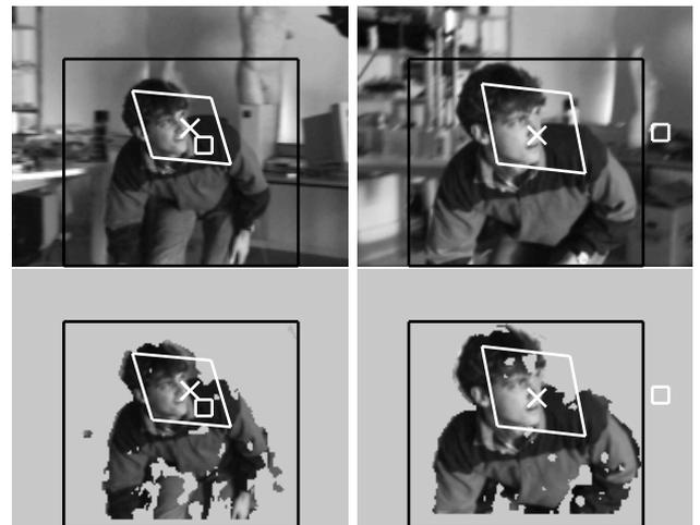
Figure 11: Pursuit during target expansion. On the top is shown the original sequence recorded during real-time pursuit, where every 12<sup>th</sup> frame is shown. In the bottom row is shown the result of the corresponding segmentation.
