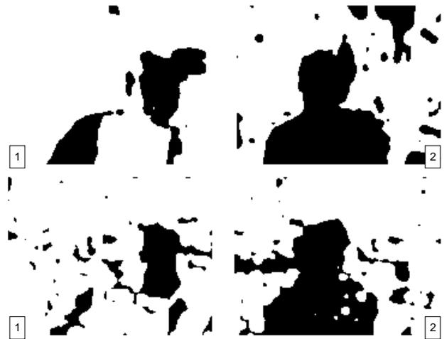
Figure 8: Motion detection (1<sup>st</sup> row) and Target segmentation (2<sup>nd</sup> row) return masks (before integration is performed) used to produce the final target masks in Figure 7 (compare with the 1<sup>st</sup> row).
