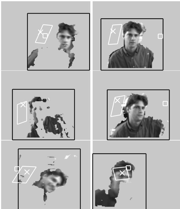
Figure 7: Resulting target pixels as extracted by the system (after integration and update) from the sequence shown in Figure 6.
