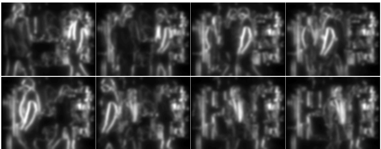
Figure 7: Certainty maps computed corresponding to the disparity map shown in Figure 6. The lighter, the higher certainty.
